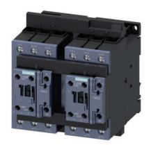
reversing contactor assembly, AC-3e/AC-3, 51 A, 22 kW / 400 V, 3-pole, 230 V AC, 50/60 Hz, screw terminal, electrical and mechanical interlock, auxiliary contacts: 2 x 1 NO
