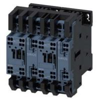
reversing contactor assembly, AC-3e/AC-3, 38 A, 18.5 kW / 400 V, 3-pole, 110 V AC, 50 Hz / 120 V, 60 Hz, spring-loaded terminal, electrical and mechanical interlock, auxiliary contacts:  $2 \times 1 \text{ NO}$
