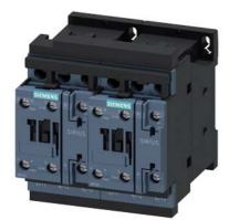
reversing contactor assembly, AC-3e/AC-3, 38 A, 18.5 kW / 400 V, 3-pole, 220 V AC, 50 Hz / 240 V, 60 Hz, screw terminal, electrical and mechanical interlock, auxiliary contacts: 2 x 1 NO
