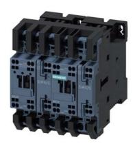
reversing contactor assembly, AC-3e/AC-3, 32 A, 15 kW / 400 V, 3-pole, 24 V DC, spring-loaded terminal, electrical and mechanical interlock, auxiliary contacts: 2 x 1 NO, with voltage tap for 3RA27
