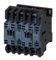
reversing contactor assembly, AC-3e/AC-3, 32 A, 15 kW / 400 V, 3-pole, 110 V AC, 50/60 Hz, spring-loaded terminal, electrical and mechanical interlock, auxiliary contacts: 2 x 1 NO
