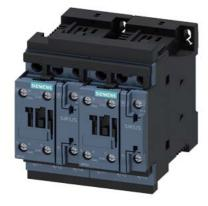
reversing contactor assembly, AC-3e/AC-3, 17 A, 7.5 kW / 400 V, 3-pole, 125 V DC, screw terminal, electrical and mechanical interlock, auxiliary contacts: 2 x 1 NO
