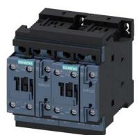
reversing contactor assembly, AC-3e/AC-3, 17 A, 7.5 kW / 400 V, 3-pole, 24 V DC, screw terminal, electrical and mechanical interlock, auxiliary contacts:  $2 \times 1 \text{ NO}$
