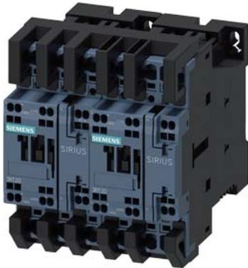
reversing contactor assembly, AC-3e/AC-3, 12 A, 5.5 kW / 400 V, 3-pole, 24 V DC, spring-loaded terminal, electrical and mechanical interlock, auxiliary contacts: 2 x 1 NO
