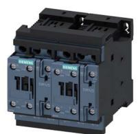
reversing contactor assembly, AC-3e/AC-3, 12 A, 5.5 kW / 400 V, 3-pole, 24 V DC, screw terminal, electrical and mechanical interlock, auxiliary contacts:  $2 \times 1 \text{ NO}$
