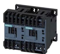
reversing contactor assembly, AC-3e/AC-3, 16 A, 7.5 kW / 400 V, 3-pole, 48 V DC, spring-loaded terminal, electrical and mechanical interlock
