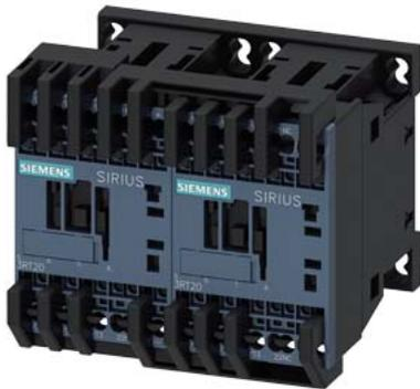
reversing contactor assembly, AC-3e/AC-3, 12 A, 5.5 kW / 400 V, 3-pole, 48 V DC, spring-loaded terminal, electrical and mechanical interlock
