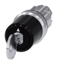
key-operated switch Siemens with key monitoring, 22 mm, round, metal shiny, lock number SSG10 with 2 keys, 3 switch positions I-O-II, latching, actuating angle 2x45°, 10:30h/12h/13:30h, key removal/ejection in O, Z=50-unit packaging
