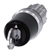
Key-operated switch IKON, 22 mm, round, metal, shiny, special lock, with 2 keys, 3 switch positions I>O<II, momentary contact type, actuating angle  $2x45^{\circ}$ , 10:30h/12h/13:30h, Key removal O
