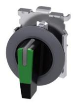
Selector switch, illuminable, 30 mm, round, Metal, matte, green, selector switch, long, front ring for flush installation, 3 switch positions I>O<II, momentary contact type, actuating angle  $2x45^{\circ}$ , 10:30h/12h/13:30h, with laser labeling, upper case
