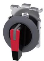
Selector switch, illuminable, 30 mm, round, Metal, matte, red, selector switch, long, front ring for flush installation, 3 switch positions I>O<II, momentary contact type, actuating angle 2x45°, 10:30h/12h/13:30h, with laser labeling, upper case
