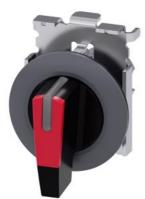
Selector switch, illuminable, 30 mm, round, Metal, matte, red, selector switch, long, front ring for flush installation, 3 switch positions I>O<II, momentary contact type, actuating angle 2x45°, 10:30h/12h/13:30h, Z=50-unit packaging
