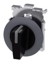
Illuminable selector switch, 30 mm, round, Metal matt, black, Selector switch short, front ring for flush installation, latching, actuating angle  $2x45^{\circ}$ , 10:30 /12 /13:30, Z=50-unit packaging
