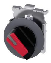
Selector switch, illuminable, 30 mm, round, Metal, matte, red, selector switch, short, front ring for flush installation, 2 switch positions O-I, latching, actuating angle 90°, 10:30h/13:30h, with laser labeling, upper case and lower case, always upper case at the beginning of the word
