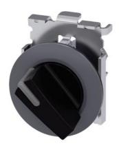
Illuminable selector switch, 30 mm, round, Metal matt, black, Selector switch short, front ring for flush installation, latching, actuating angle 90°, 10:30 /13:30, Z=50-unit packaging
