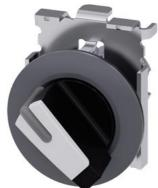
Selector switch, illuminable, 30 mm, round, Metal, matte, white, selector switch, short, front ring for flush installation, 2 switch positions O<I, momentary contact type, Actuating angle 45°, 10:30h/12h, with laser labeling, upper case and lower case, always upper case at the beginning of the word
