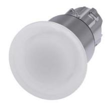
Illuminated mushroom pushbutton, 22 mm, round, metal, shiny, white, 40 mm, 3 switch positions, after pushing in Retraction to center position, after pulling out the button Retraction to center position, with laser labeling, upper case
