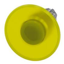
Illuminated mushroom pushbutton, 22 mm, round, metal, shiny, yellow, 60 mm, latching, pull-to-unlatch mechanism, with laser labeling, upper case
