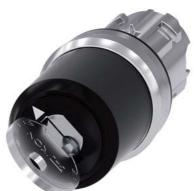
Key-operated switch IKON, 22 mm, round, metal, shiny, lock number 360012K1, with 2 keys, 2 switch positions O-I, latching, actuating angle 90°, 10:30h/13:30h, key removal O+I, with laser labeling, inscription or symbol Customer-specific selection with SIRIUS ACT configurator (CIN)
