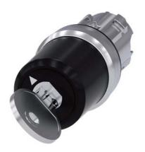
Key-operated switch BKS, 22 mm, round, metal, shiny, lock number S1, with 2 keys, 2 switch positions O-I, latching, actuating angle  $90^\circ$ , 10:30h/13:30h, key removal I, Z=50-unit packaging
