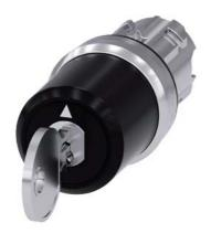
key-operated switch Siemens, 22 mm, round, metal, shiny, lock number SSG10, with 2 keys, 3 switch positions I-O-II, latching, actuating angle  $2x45^{\circ}$ , 10:30h/12h/13:30h, key removal I+II, Z=50-unit packaging
