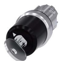
key-operated switch Siemens, 22 mm, round, metal, shiny, lock number SSG10, with 2 keys, 2 switch positions O-I, latching, actuating angle 90°, 10:30h/13:30h, key removal O, with laser labeling, upper case
