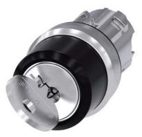
RONIS key-operated switch, 22 mm, round, metal, shiny, lock number 455, with 2 keys, 2 switch positions O-I, latching, actuating angle  $90^\circ$ , 10:30h/13:30h, key removal O, with laser labeling, lower case
