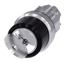
RONIS key-operated switch, 22 mm, round, metal, shiny, lock number 455, with 2 keys, 2 switch positions O<I, momentary contact type, Actuating angle 45°, 10:30h/12h, key removal O, with laser labeling, inscription or symbol Customerspecific selection with SIRIUS ACT configurator (CIN)
