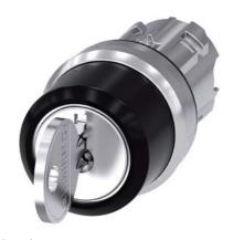
RONIS key-operated switch, 22 mm, round, metal, shiny, special lock, with 2 keys, 3 switch positions I>O<II, momentary contact on the left, latching on the right, actuating angle 2x45°, 10:30h/12h/13:30h, Key removal O+II, possible special locks: SB31, 421, 455
