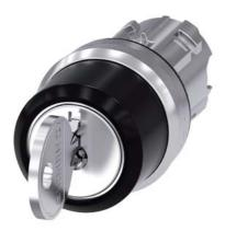
RONIS key-operated switch, 22 mm, round, metal, shiny, special lock, with 2 keys, 3 switch positions I-O<II, left latching, right momentary contact type, actuating angle 2x45°, 10:30h/12h/13:30h, key removal O+I, possible special locks: SB31, 421, 455
