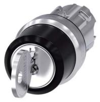
RONIS key-operated switch, 22 mm, round, metal, shiny, lock number SB30, with 2 keys, 3 switch positions I-O<II, left latching, right momentary contact type, actuating angle  $2x45^{\circ}$ , 10:30h/12h/13:30h, key removal O+I, possible special locks: SB31, 421, 455, Z=50-unit packaging
