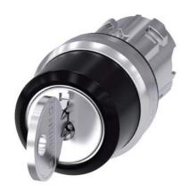
RONIS key-operated switch, 22 mm, round, metal, shiny, special lock, with 2 keys, 3 switch positions I-O-II, latching, actuating angle  $2x45^{\circ}$ , 10:30h/12h/13:30h, key removal O+I, possible special locks: SB31, 421, 455
