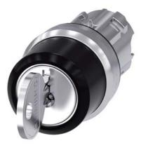
RONIS key-operated switch, 22 mm, round, metal, shiny, lock number SB30, with 2 keys, 3 switch positions I-O-II, latching, actuating angle 2x45°, 10:30h/12h/13:30h, Key removal II, possible special locks: SB31, 421, 455, with laser labeling, lower case
