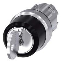
RONIS key-operated switch, 22 mm, round, metal, shiny, lock number SB30, with 2 keys, 3 switch positions I-O-II, latching, actuating angle 2x45°, 10:30h/12h/13:30h, Key removal II, possible special locks: SB31, 421, 455, with laser labeling, upper case and lower case, always upper case at beginning of line
