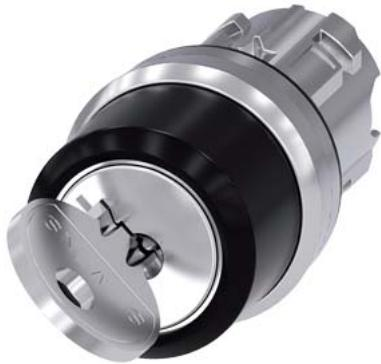
RONIS key-operated switch, 22 mm, round, metal, shiny, lock number SB30, with 2 keys, 2 switch positions O-I, latching, actuating angle 90°, 10:30h/13:30h, key removal O, possible special locks: SB31, 421, 455, Z=50-unit packaging
