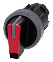
Selector switch, illuminable, 22 mm, round, plastic with metal front ring, red, selector switch, short, 3 switch positions I-O<II, left latching, right momentary contact type, actuating angle 2x45°, 10:30h/12h/13:30h, with laser labeling, inscription or symbol Customer-specific selection with SIRIUS ACT configurator (CIN)
