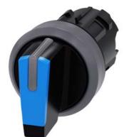
Selector switch, illuminable, 22 mm, round, plastic with metal front ring, blue, selector switch, short, 3 switch positions I>O<II, momentary contact type, actuating angle 2x45°, 10:30h/12h/13:30h, with laser labeling, upper case and lower case, always upper case at beginning of line
