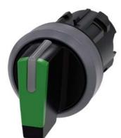
Selector switch, illuminable, 22 mm, round, plastic with metal front ring, green, selector switch, short, 3 switch positions I>O<II, momentary contact type, actuating angle 2x45°, 10:30h/12h/13:30h, Z=50-unit packaging
