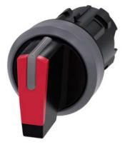
Selector switch, illuminable, 22 mm, round, plastic with metal front ring, red, selector switch, short, 3 switch positions I>O<II, momentary contact type, actuating angle 2x45°, 10:30h/12h/13:30h, with laser labeling, upper case and lower case, always upper case at the beginning of the word
