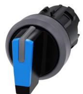
Selector switch, illuminable, 22 mm, round, plastic with metal front ring, blue, selector switch, short, 3 switch positions I-O-II, latching, actuating angle 2x45°, 10:30h/12h/13:30h, with laser labeling, upper case and lower case, always upper case at the beginning of the word
