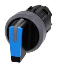
Selector switch, illuminable, 22 mm, round, plastic with metal front ring, blue, selector switch, short, 3 switch positions I-O-II, latching, actuating angle 2x45°, 10:30h/12h/13:30h, with laser labeling, upper case
