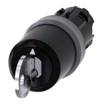
Key-operated switch IKON, 22 mm, round, plastic with metal front ring, lock number 360012K1, with 2 keys, 3 switch positions I-O-II, latching, actuating angle 2x45°, 10:30h/12h/13:30h, key removal O, with laser labeling, upper case
