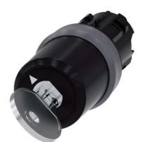
Key-operated switch BKS, 22 mm, round, plastic with metal front ring, lock No. E9 (VW), without key, 2 switch positions O-I, latching, actuating angle 90°, 10:30h/13:30h, key removal O, with laser labeling, inscription or symbol Customer-specific selection with SIRIUS ACT configurator (CIN)
