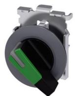
Selector switch, illuminable, 30 mm, round, Metal, matte, green, selector switch, long, front ring for flush installation, 2 switch positions O<I, momentary contact type, Actuating angle 45°, 10:30h/12h, with laser labeling, inscription or symbol Customer-specific selection with SIRIUS ACT configurator (CIN)
