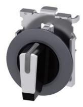
Selector switch, illuminable, 30 mm, round, Metal, matte, white, selector switch, short, front ring for flush installation, 3 switch positions I>O<II, momentary contact type, actuating angle 2x45°, 10:30h/12h/13:30h, with laser labeling, inscription or symbol Customer-specific selection with SIRIUS ACT configurator (CIN)
