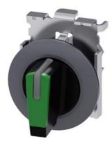
Selector switch, illuminable, 30 mm, round, Metal, matte, green, selector switch, short, front ring for flush installation, 3 switch positions I>O<II, momentary contact type, actuating angle  $2x45^{\circ}$ , 10:30h/12h/13:30h, with laser labeling, upper case
