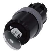
Key-operated switch BKS, 22 mm, round, plastic with metal front ring, Lock No. E2 (VW), without key, 2 switch positions O-I, latching, actuating angle  $90^\circ, 10:\!30h/13:\!30h,$  key removal O, Z=50-unit packaging
