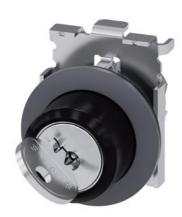
RONIS key-operated switch, 30 mm, round, Metal, matte, front ring for flush installation, lock number SB30, with 2 keys, 2 switch positions O-I, latching, actuating angle 90°, 10:30h/13:30h, key removal I, possible special locks: SB31, 421, 455, with laser labeling, upper case
