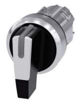
Selector switch, illuminable, 22 mm, round, metal, shiny, white, selector switch, long, 3 switch positions I>O<II, momentary contact type, actuating angle 2x45°, 10:30h/12h/13:30h, Z=50-unit packaging
