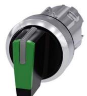
Selector switch, illuminable, 22 mm, round, metal, shiny, green, selector switch, short, 3 switch positions I-O<II, left latching, right momentary contact type, actuating angle 2x45°, 10:30h/12h/13:30h, Z=50-unit packaging
